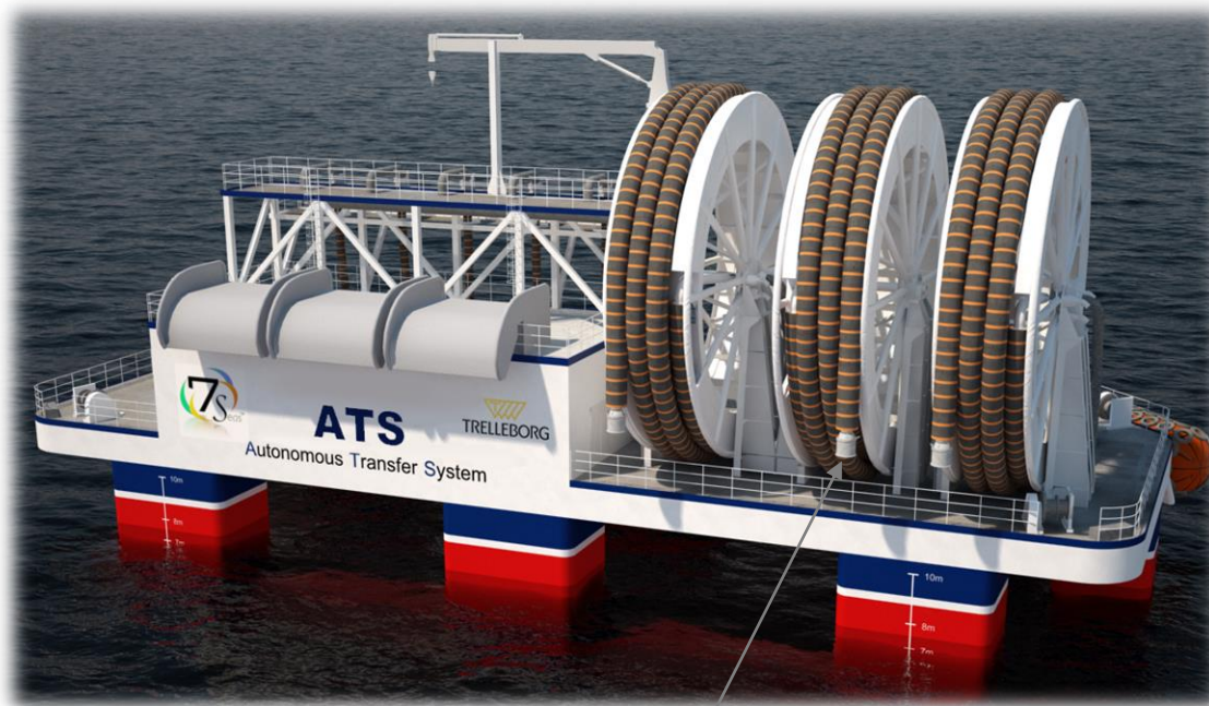
LNG Hoses disconnected from Shore Connection
